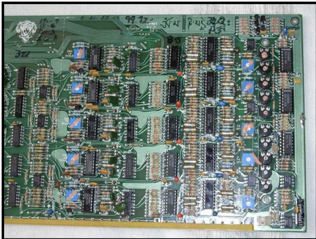
Figure 8: The voice board of the Prophet 5 with CEM chips (Picture source: http://users.telenet.be/prophet-5 )
