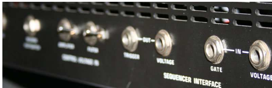
Figure 3: Gate, CV, Trigger and Filter Inputs at the back of the Prophet 5
